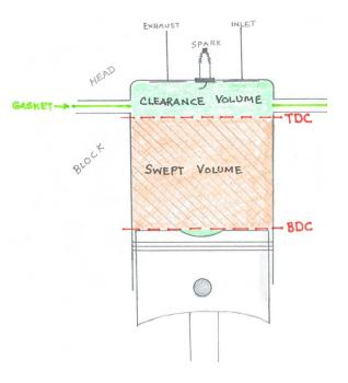
There were two variants of Combustion Chamber volume. On 18G series engines the cylinder heads had 43cc combustion chambers and they had 6.2cc dished pistons. The 18V series engines had cylinder heads with smaller 39cc combustion chambers with 16.2cc dished pistons. The volume caused by the standard gasket thickness is about 3.2cc and the volume between TDC and the block deck is usually about 5.1cc.
