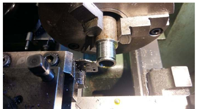
Photo 3 – making the EN16 squeeze clip.
