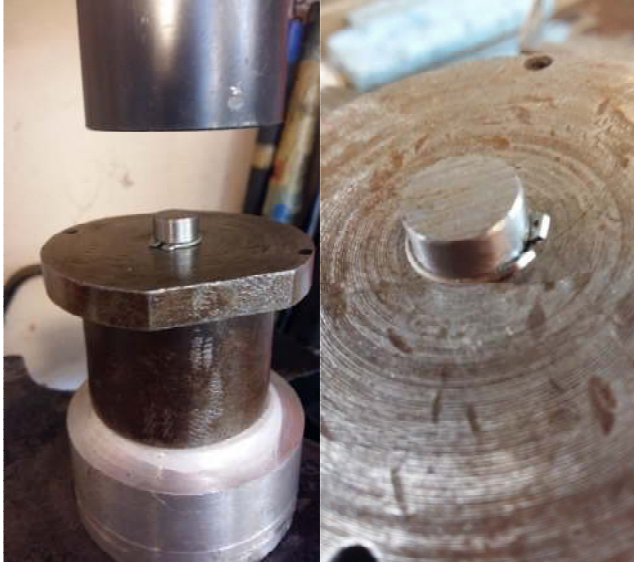
Photo 4 shows the replacement circlip about to receive some metallic torture and photo 5 shows that it didn't submit!
