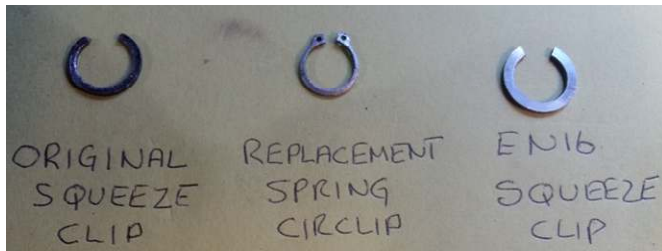
Photo 1 – the EN16 squeeze clip was made by the author (Eric Worpe) and is referred to later in this article.
