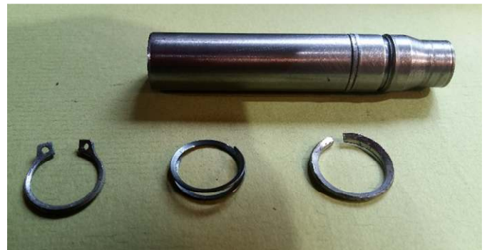
Photo 8 – shows the three tested clips and the dummy shaft.
