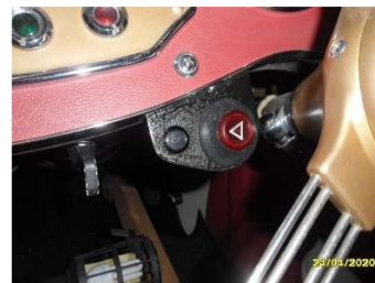
Picture shows the Durite switch installed in a TD. The small indicator next to it is a low oil pressure warning not yet connected.
