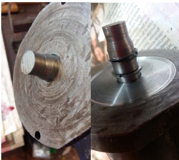
Photo 6 shows that the Pelton Retaining Ring withstood the force, but the EN16 "squeeze in" clip shown on the right in photo 7, didn't.
