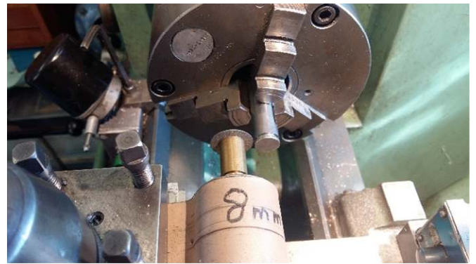
Photo 2 – deepening the groove.
