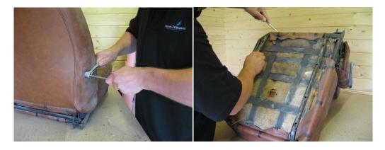
Now, remove the spring steel clips which hold the upholstery to the framework, this will allow the cover to be pulled off the seat. After removing the clips temporarily fit the chrome adjuster handle and open the seat up fully. The open seat will now allow you to grasp the flap of material and pull from the slot in the seat, once done the upholstery can then be slid off being careful over the adjuster shaft.
