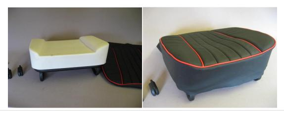
Mark the position of the front edge of the seat upholstery on the front lower edge of the base frame pipe. This will give a reference point for assembly. Failure to do this may lead to the upholstery not matching after fitment.
