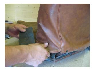
Glue should now be applied to the inner face of the back foam and the surface of the inner upholstery, if you are using contact adhesive allow enough time for the adhesive to set before commencing to assemble.
