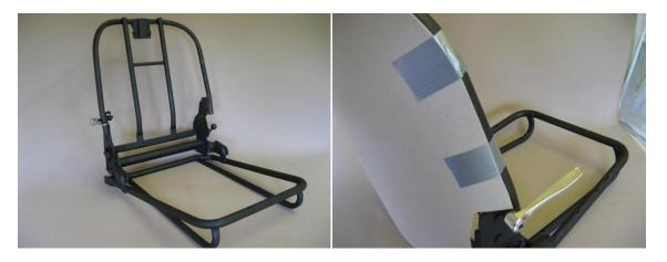
Here is the seat back frame with new back foam installed; the foam is simply glued into place with contact adhesive. We recommend using duck tape to assist with holding the foam in place to contour of the frame whilst the adhesive cures.
