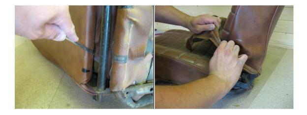
The seat upholstery is removed using the same method; care should taken when prying off the clips as the ends are barbed and carelessly prying them off will damage the upholstery.
