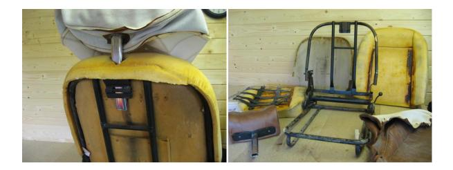
The seat and back frame should now be undone and the parts separated for cleaning and renovation.
